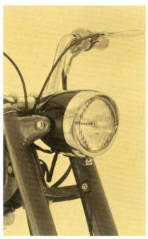
SAFETY PLUS – Full front-and-rear lighting, dual-shoe brakes, famous Pirelli tires, welded tubular steel frame and 2.50 x 17" wheels with ball-bearing hubs all provide you with the extra margin of safety you can always expect from Harley-Davidson.
