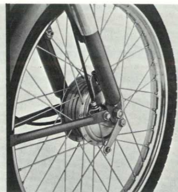
Both front and rear wheels have full-width hubs for extra strength and braking power
